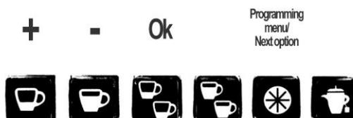
First press "Ok" and then it will appear the current time and day of the week. The blinking value of the hours can be modified with the + or – keys. When the right value is settled, you can press Ok to accept and the minutes will start to blink. Select again the right value with + and – and press Ok when the desired minutes are settled. Finally, set the day of the week the same way, pressing Ok to accept it.
