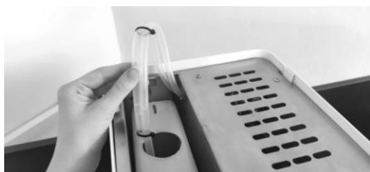
5. Remove the tank and fill with water.
