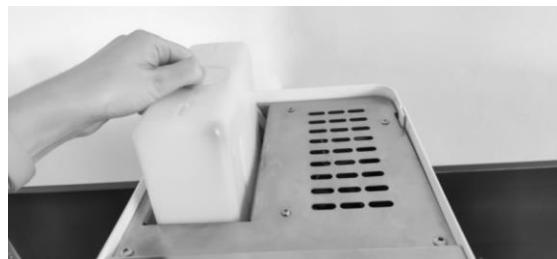
6. Reinsert the tank. Make sure that the end of the filter is submerged at the bottom of the tank.
